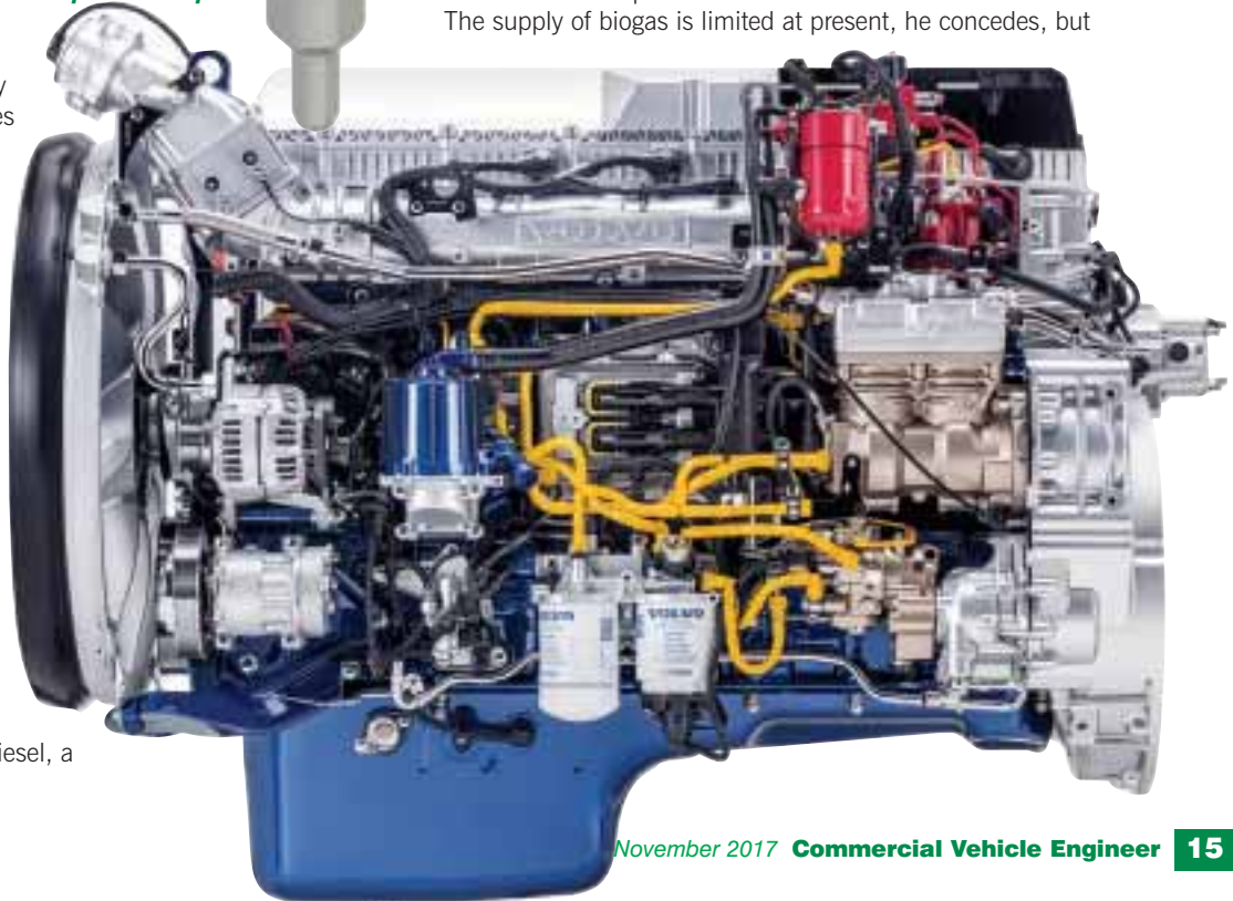
Largely unchanged diesel engine running on gas: thanks to this clever injector from Westport and Delphi.
